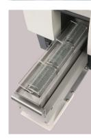
The load vessel accepts up to 60 slides and can be filled with reagent – increases throughput and allows for wet or dry coverslipping.
